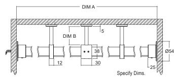
/CPD - Double coupler. See page 3 for details. Specify Dim A, B and C
